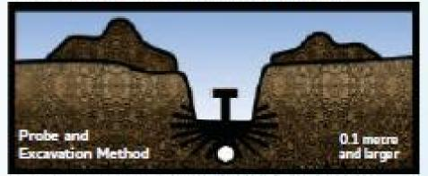
In addition to other excavation methods previously mentioned, a probe and excavate technique can be used for gas pipelines 0.1 metre and larger in diameter.
