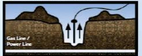
Only oscillating head type nozzles are to be used for the water wand. When excavating within 1 metre horizontally of a marked line the maximum settings of 38°C water temperature and 10.340 Kpa (1.500 psi) must not be exceeded. The end of the vacuum tube shall be neoprene or equivalent. Expose the buried line by using a SWEEPING MOTION ONLY, perpendicular to the locate markings, uncli the line is sighted. After sighting, the line shall not be contacted by spray or vacuum.
