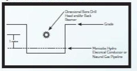
Figure 3: Observation Hole - Profile View
