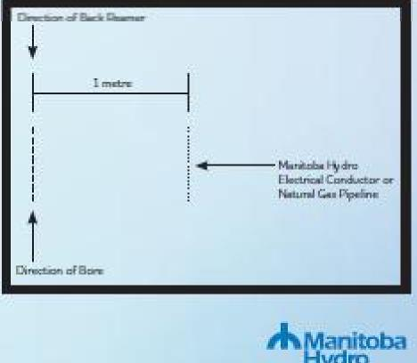
Figure 5: Drilling Parallel to Manitoba Hydro Conductors and Natural Gas Pipelines - Profile View
